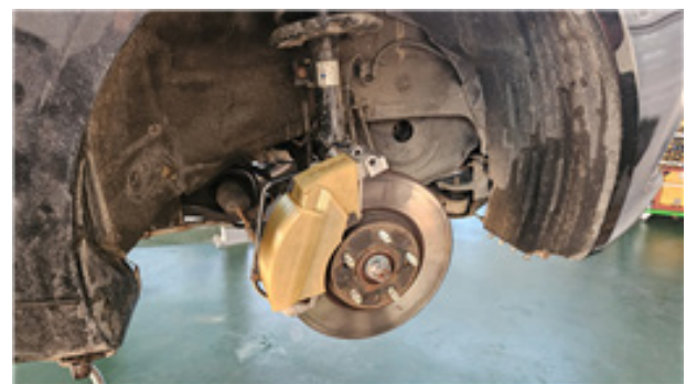
Fig. 2 BWPs emission reduction device installation on real-vehicle brake system
