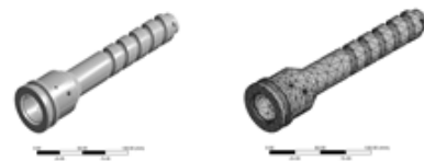
Fig. 1 Shape simplification and meshing of WAM gear
