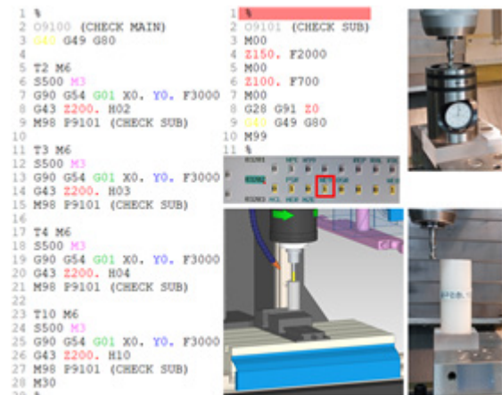
Fig. 3 Setting verification for real machining
