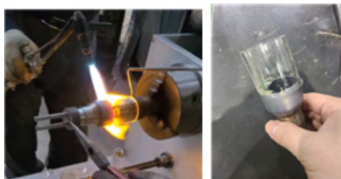
Fig. 3 Bonding process for glass tube and Kovar metal
