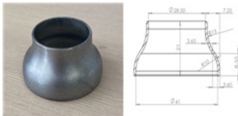
Fig. 1 The photograph and drawing of Kovar metal
