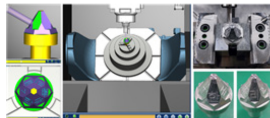
Fig. 4 Simulation, 5-axis machining and results
