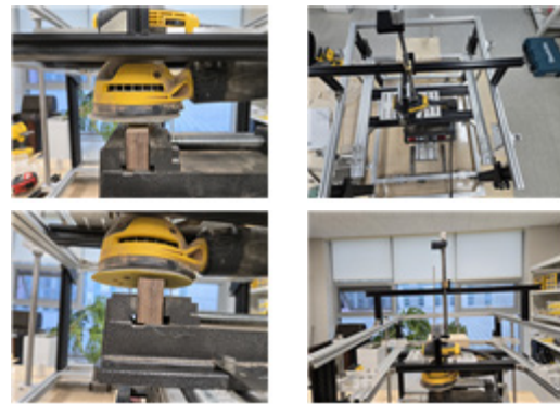
Fig. 1 Custom sanding apparatus with detachable handheld sander
