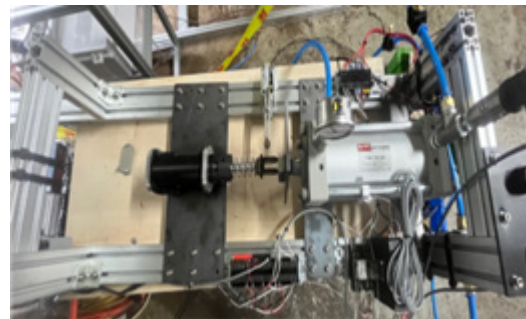
Fig. A actuator for a damper test
