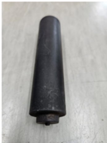
Pin \Phi 3 / Shoulder \Phi 15
